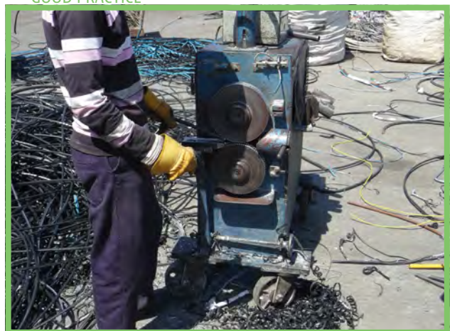
Cable stripper avoiding air pollution (Morocco) ©Empa
