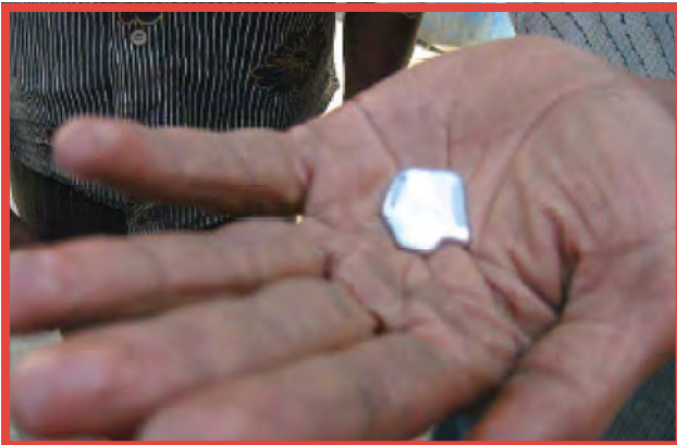
Mercury used for amalgamation to recover gold ©Empa
