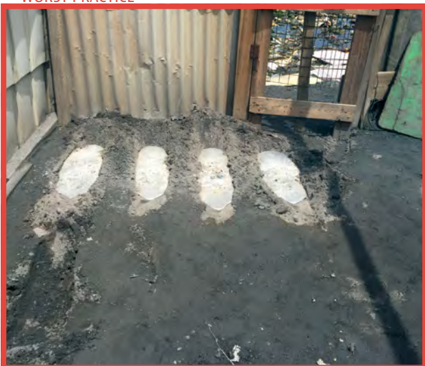
Aluminium ingots produced in open soils (Ghana) ©WRF
