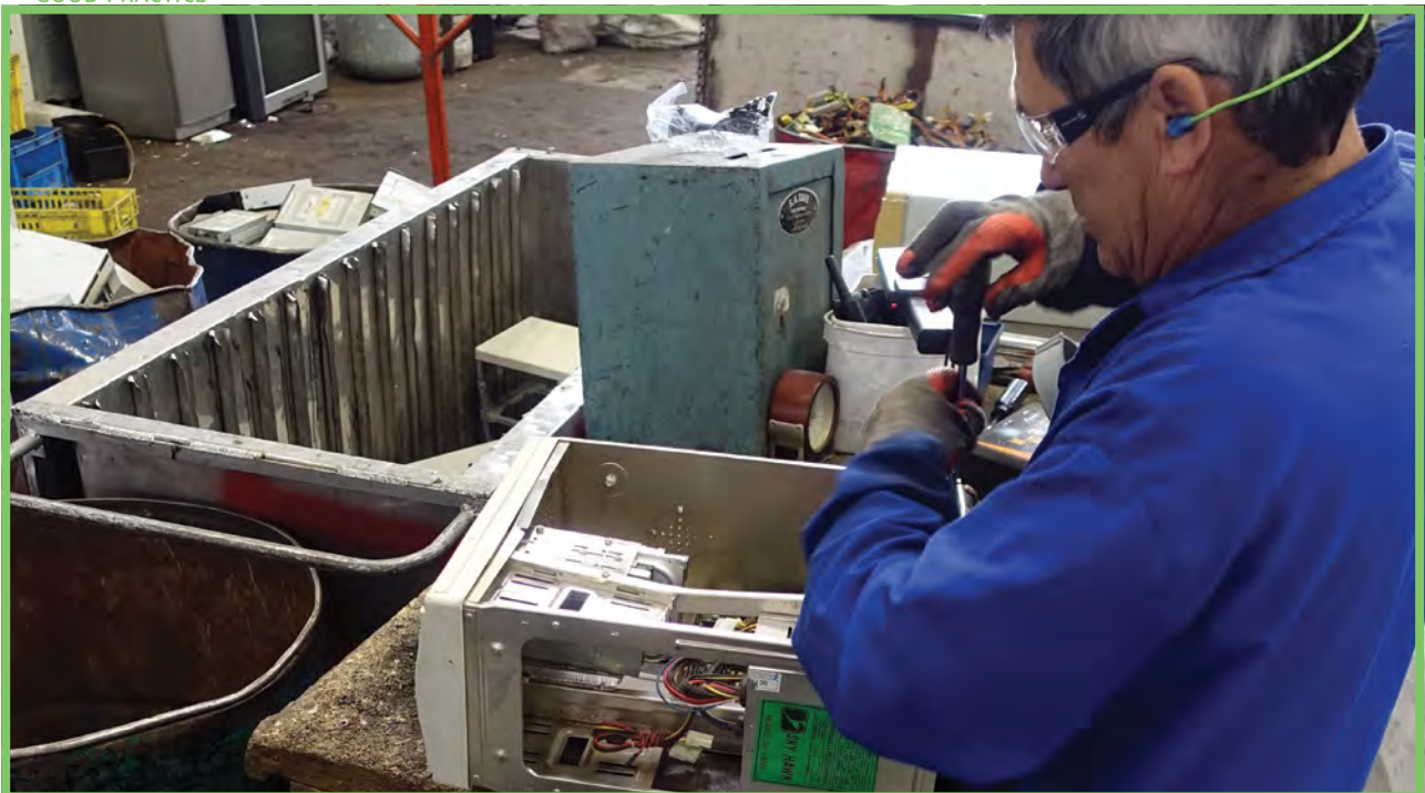
Safe manual dismantling of end-of-life computers to separate materials containing precious metals (e.g. circuit boards) and copper, to be sent to a licensed metallurgical processing facility ©WRF
