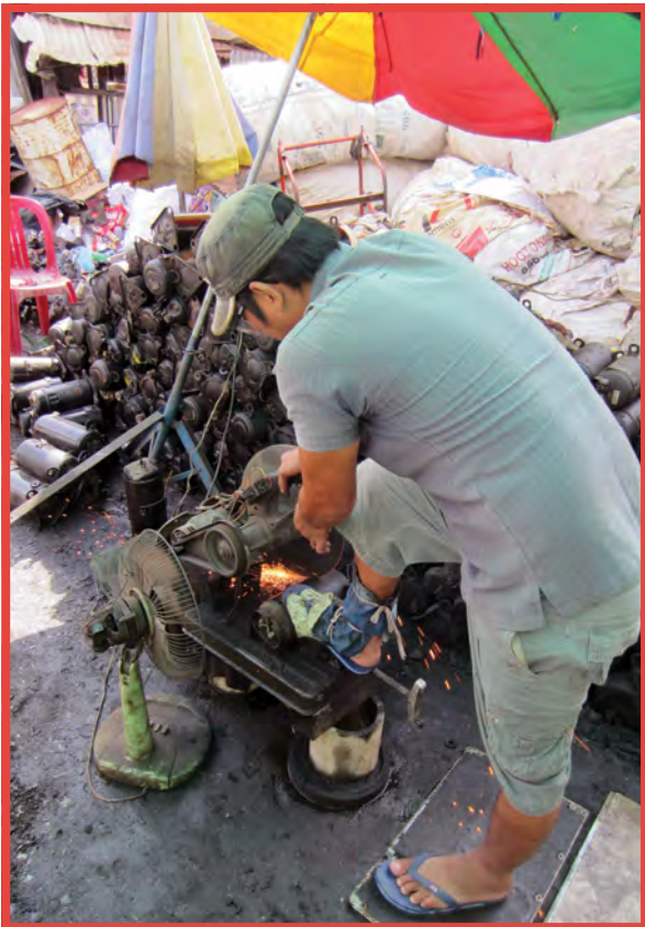
Worker with no protection sawing scrap fridge compressors resulting in soil pollution from used oil (Cambodia) ©WRF
