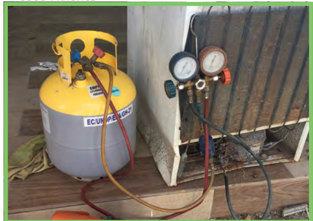
Extraction of cooling gases before fridge dismantling for recycling (Ghana) ©WRF
