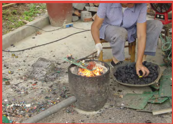
De-soldering of a motherboard in China ©Empa
