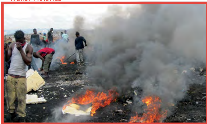
'Fuelling the fire' with highly flammable fridge insulation materials to recover metals in Agbogbloshie, Accra, Ghana ©Oeko Institut
