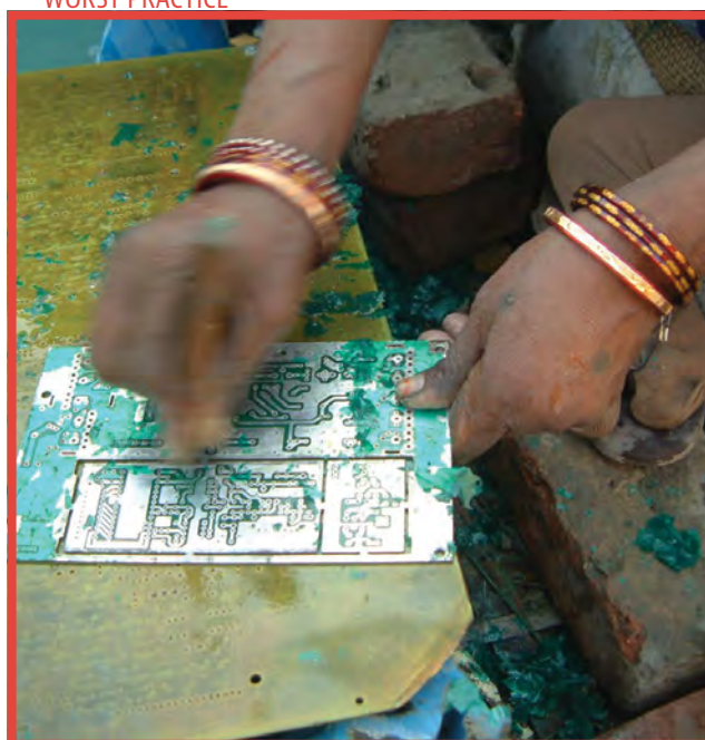
Preparation for sulphuric acid baths to recover copper from printed circuit boards ©Empa
