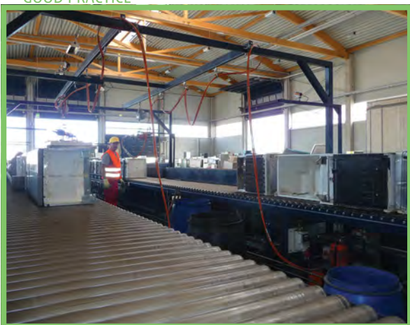
Properly functioning fridge components disassembly line, Switzerland ©Empa
